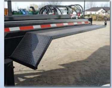
Skid proof front fenders (steel - checker plate).
