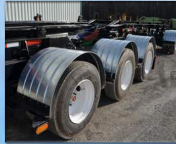
Stainless steel grooved fenders.
