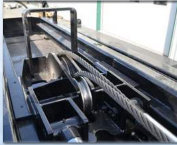
Sliding carriage on Nylatron wear pads.
