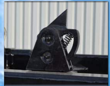
Heavy-duty spring-loaded container push-out (optional).
