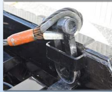
1" hoist cable (6 x 26 - 106,000 lb. capacity) with D-ring for greater versatility and resistance.
