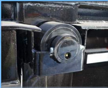
Greasable side rollers with bronze aluminum bushing.
