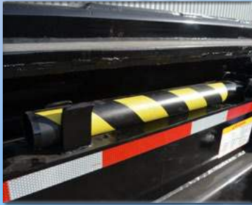
Steel props for safe maintenance.
