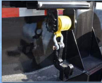
Container hooks and straps (compliant with CCS norm 10).
