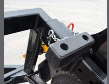
Protective pads prevent damage to container.
