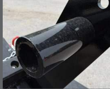
Movable stoppers to accommodate multiple container sizes.
