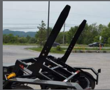
1/2" to 1" steel forks for container pick up.
