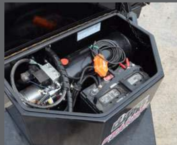
12V hydraulic unit - wired remote control, deep cycle battery and charger.
