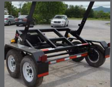
1 coat of epoxy primer and two coats of black urethane paint.
