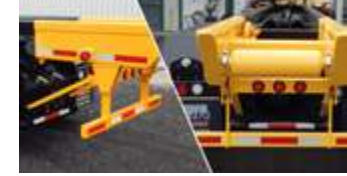
Auto-Retract mechanical ICC Bumper.
