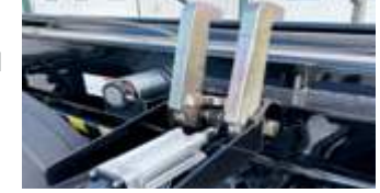
Pneumatic lock system (air hooks) zinc plated, saving.
