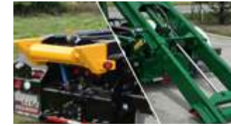
Optional 100,000 lb. steel extendable hydraulic tail (stinger tail).
