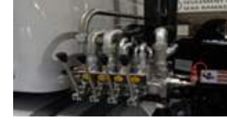
Zinc plated SALAMI 37 GPM manual controls for hydraulic operations (outside cab).
