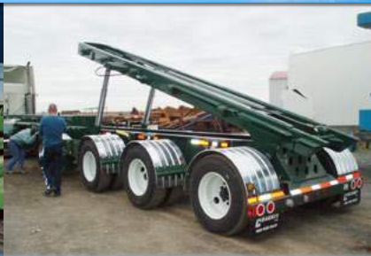
Wide cylinder footing adds overall rigidity and stability to the lift system.
