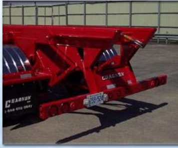
Retractable bumper for conventional trailer tail.
