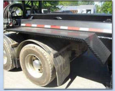
Skid proof front fenders (steel - checker plate).
