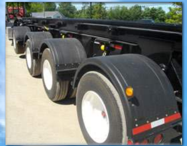
Multiple configurations possible with two, three, four or more axles.
