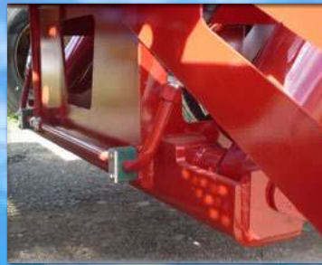
Wide cylinder footing adds overall rigidity and stability to the lift system.
