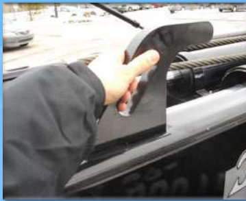
Moveable container stoppers with heavy-duty pockets.
