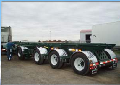
Moveable container stoppers with heavy-duty pockets.
