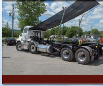
Hydraulic tarping system with telescopic arms and masts (optional).
