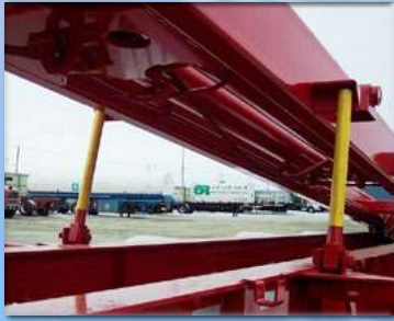
Steel props for safe maintenance.
