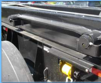
Flat plates between rollers for better support and an easier glide.
