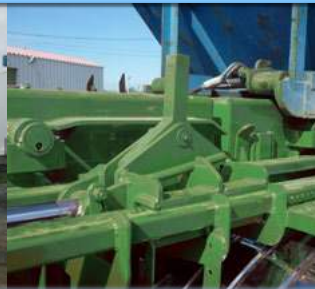
Flat plates between rollers for better support and an easier glide.
