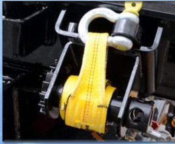
Load binder winch and hook, (NSC - norm 10 compliant).
