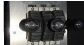
In-cab heavy duty ergonomic air over hydraulic controls.
