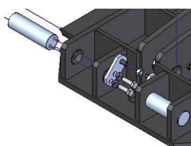
**Sliding carriage reeving cylinder attachment**
